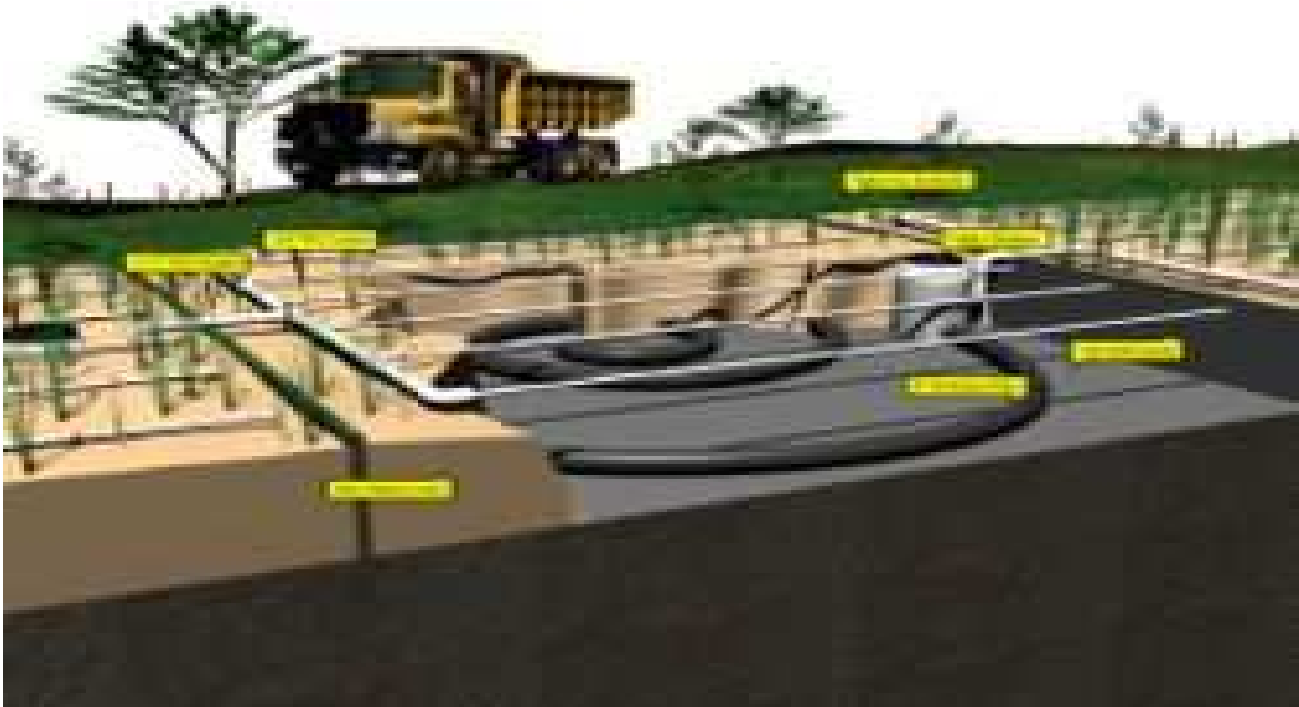
Photo 13.1 Vertical Flow Constructed Wetlands
